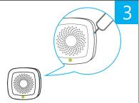
According to the APP tip, long press the device networking key 2 seconds later, the green light flash, APP interface appears tips, networking success. (The blue dots shown in the graph is the position of the device network key, green dot is the network status lamp.)
