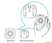
Note that the mounting base shall be up as the direction of arrow shown in the graph. Finally, hang the detector into the mounting base.
