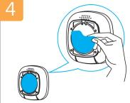
Tear off the gummed film, stick the equipment in the required area.
