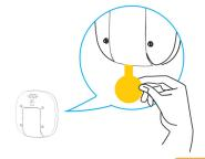
Remove battery insulation film to power on.
